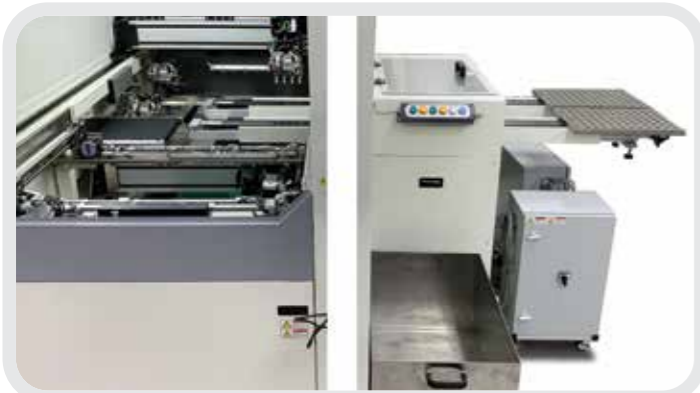
Dual Bridge Axis – Example Offload Configuration
