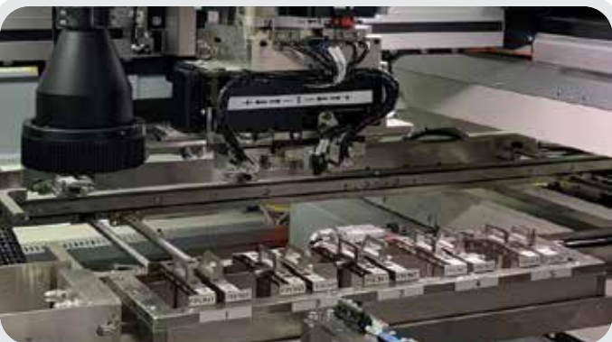
Servo Gripper and Auto Finger Change
